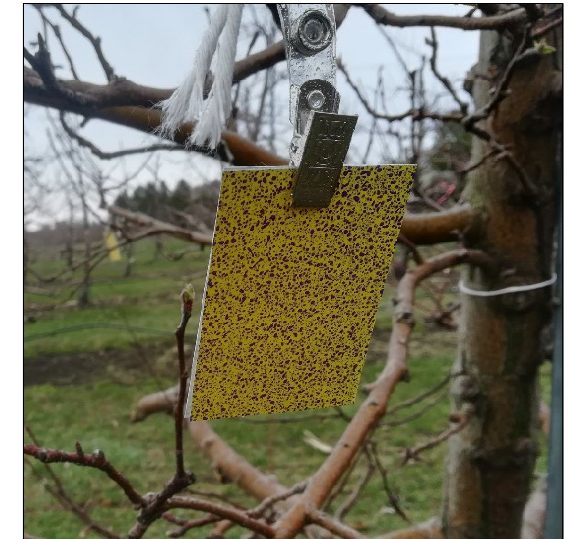
Figure 2. Water-sensitive paper card (for quantifying spray coverage) in an apple tree after a spray application.
