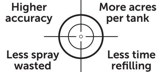
► Because it uses less spray volume per acre, the sprayer can spray more acres per tank of mixture, thus reducing tank refilling times.
