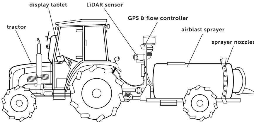
► The Intelligent Sprayer is a modified airblast pesticide sprayer that uses the same LiDAR technology as driverless cars. But instead of seeing the road, the sprayer can see the size and depth of orchard tree canopies. With this laser-guided technology, the Intelligent sprayer system can minimize spray drift and save farmers on pesticide costs.
